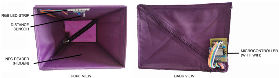
Fig. 2. Front and back view of the augmented shoe box.
