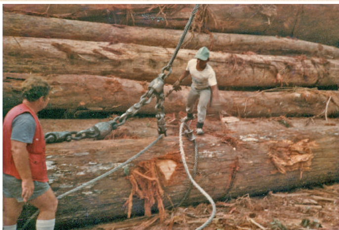
Fig.10: Log deck and close up of Butt-Rigging for High Lead Operation, c. 1978. (Photographer unknown; author's camera) The choker setter is tightening a loose shackle pin on the mainline swivel. The standard Young butt-rigging consisting of two or three mainline swivels and together with drop swivels, chokers etc. as shown here, weighed half a ton. In addition to providing the strength to withstand continuous heavy loads safely this ensured that it dropped to the ground and did not hang up in tree canopies on the outhaul.
