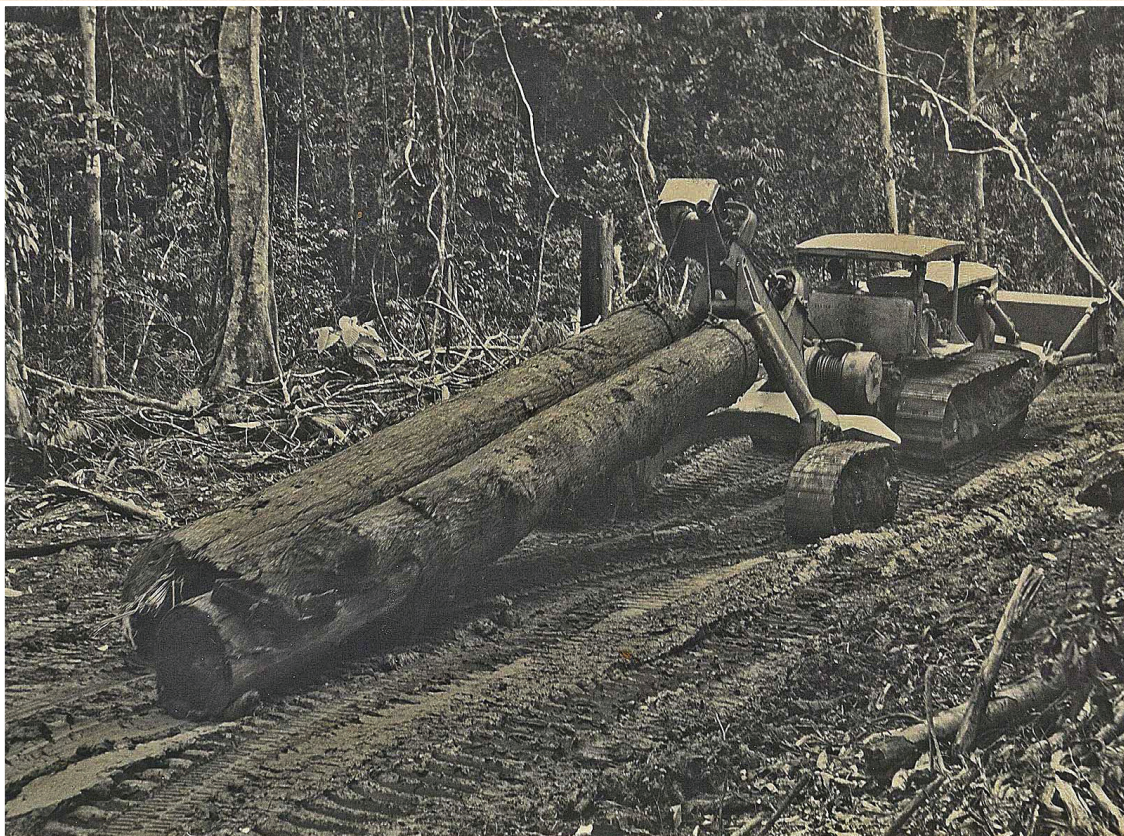
Fig.1 : Caterpillar D8 with Hyster Logging Arch, North Borneo Timbers, Kretam 1951. (Photo: George Brown, author's collection.)
