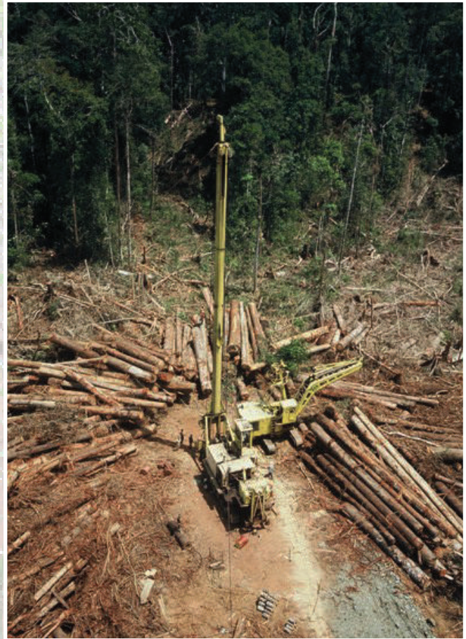
Fig. 17: Madill track-mounted mobile tower, Sabah Timbers, Tinkayu. (Photo R.M. Macpherson collection)
