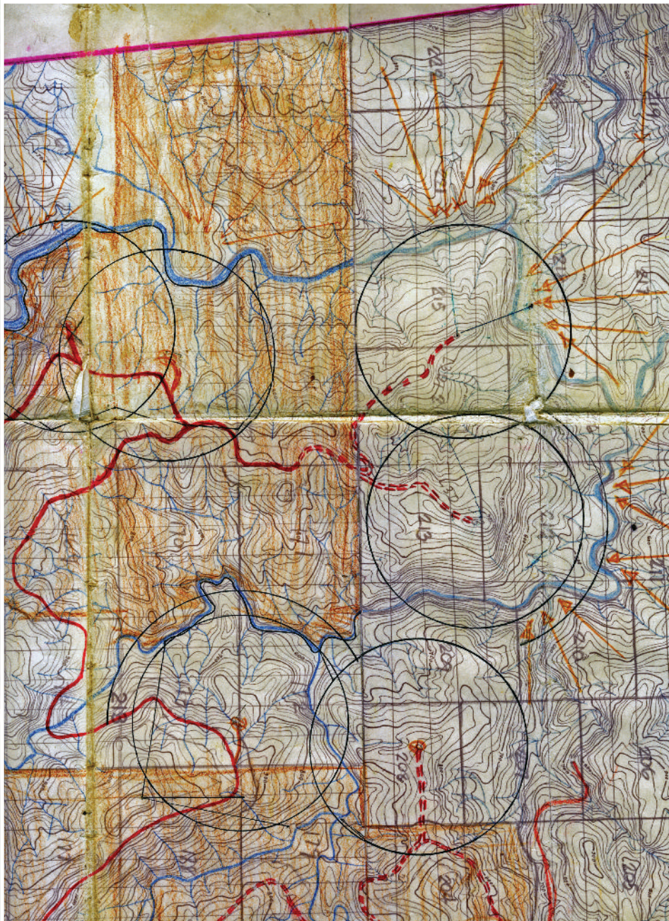
Fig.7: Map to scale of 1:10,000 of part of North Borneo Timbers workings c.1978. (Author's working plan) Yarder settings are shown by circles with tractor feed indicated by arrows.
