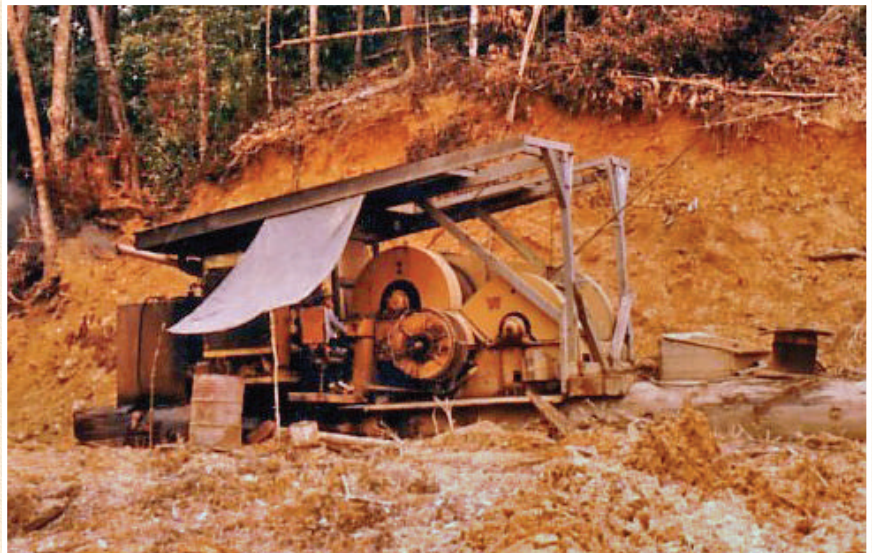
Fig.8: Washington 227 sled-mount yarder, North Borneo Timbers c. 1978. (Photo Ross Ibbotson). The yarder is located about 100ft from the base of the spar tree with the main line running up to the block at an angle of 45°.
