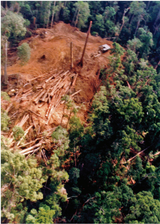
Fig. 16: Aerial view of yarder operating on remote setting; North Borneo Timbers c.1980 (Photo Ross Ibbotson) The yarder is decking a big log while the skidder can just be seen leaving the deck to the left.
