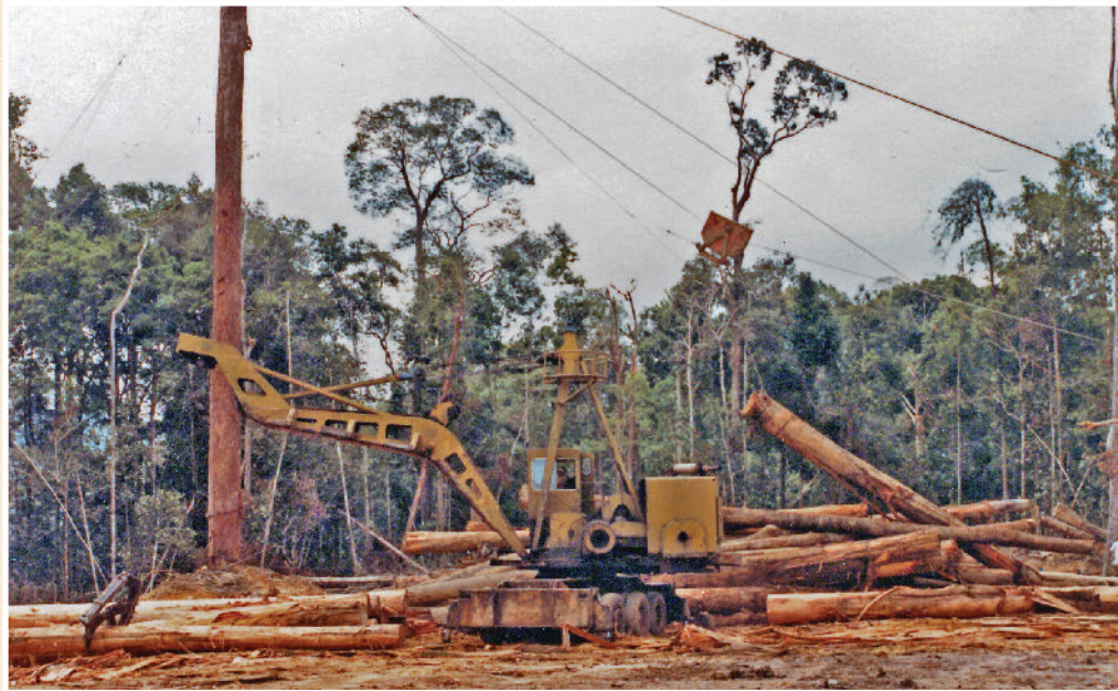
Fig. 14: Decking Scooter turn; North Borneo Timbers c. 1978. (Photo Ross Ibbotson) The logs are being cleared and prepared for loading by a Washington TL-6 grapple loader. With the high output of a scooter set up the landings could easily become congested and needed a loader in attendance.
