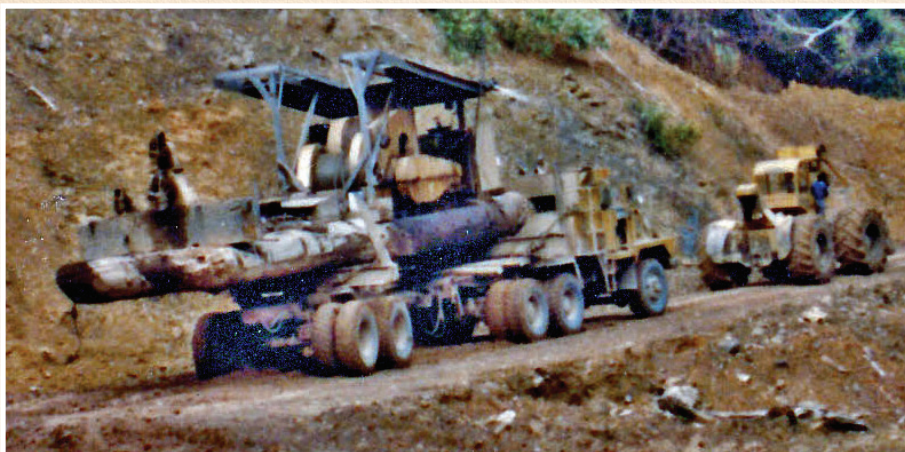
Fig.5: Washington 227 yarder carried by a Pacific P16 logging truck getting a helping hand from a Clark 668 log skidder, North Borneo Timbers, Brumas c. 1980. (Photo Ross Ibbotson) Note wear on front of runners.
