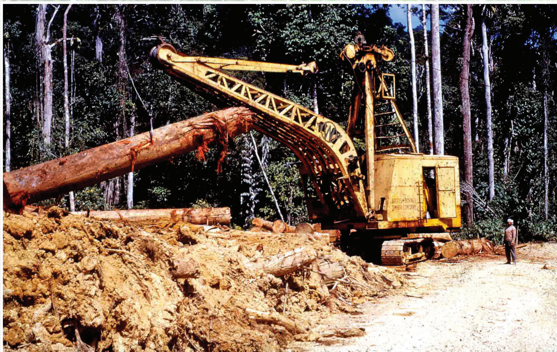
Fig.2: Washington Iron Works TL-15 with guy-lines rigged for yarding: British Borneo Timbers, Kalumpang, 1958. (Photo Keith Wookey; Robin Wookey collection).
