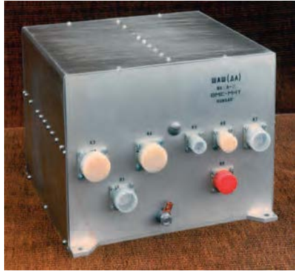
SAS (Signal Analyser and Sampler) plasma wave experiment, ELTE Space Research Group, 1989
