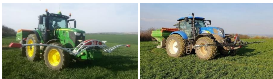
Figure 1 Nitrogen application by crop sensing system Fritzmeier ISARIA (left) and AgLeader OptRx (right) on the field. Photo by J. Mezera
