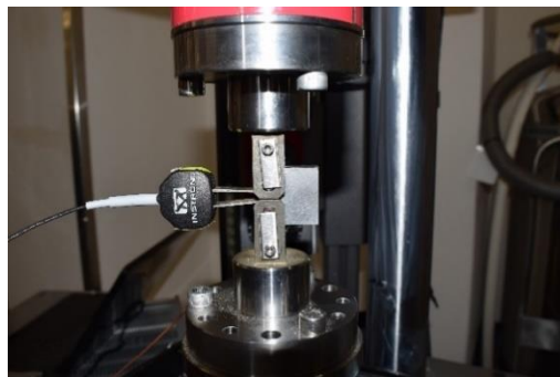
Figure 2 Testing of CT sample using machine extensometer Instron Electropuls E 10000
