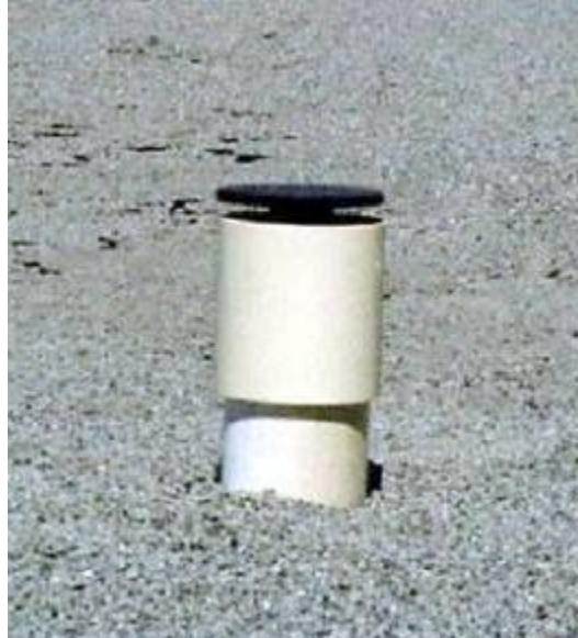
Fig. 2 Cox sand catcher ( www.sensit.com )
