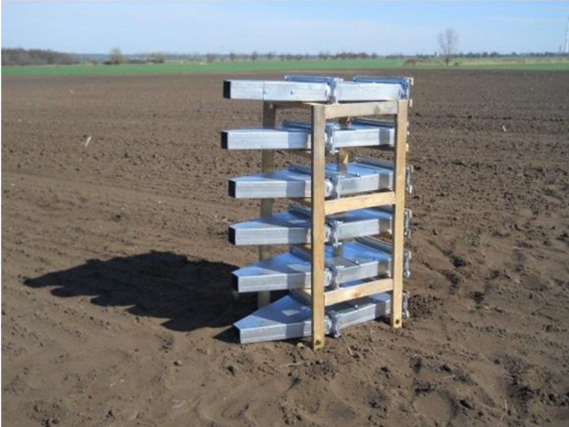
Fig. 10 Soil particle catcher devices (Lackóová et al., 2013)
