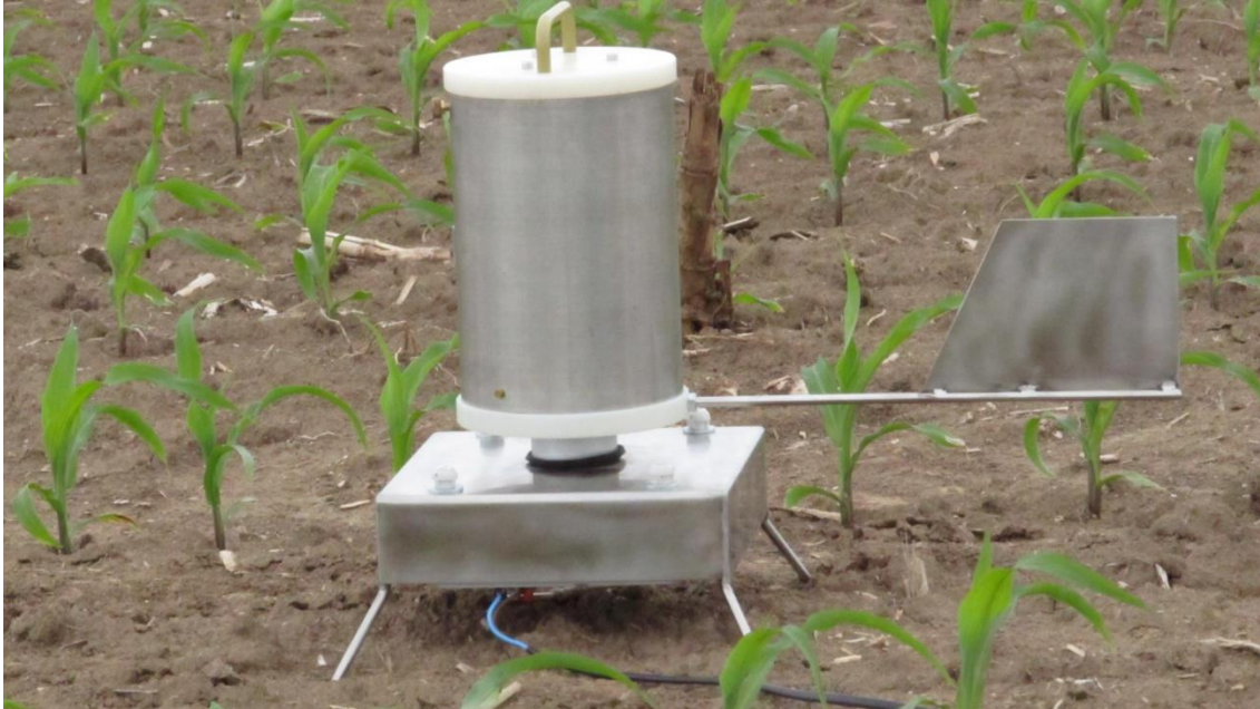
Fig. 9 Deflameter with active trap soil particles and time recording (Krmelová et al., 2012)
