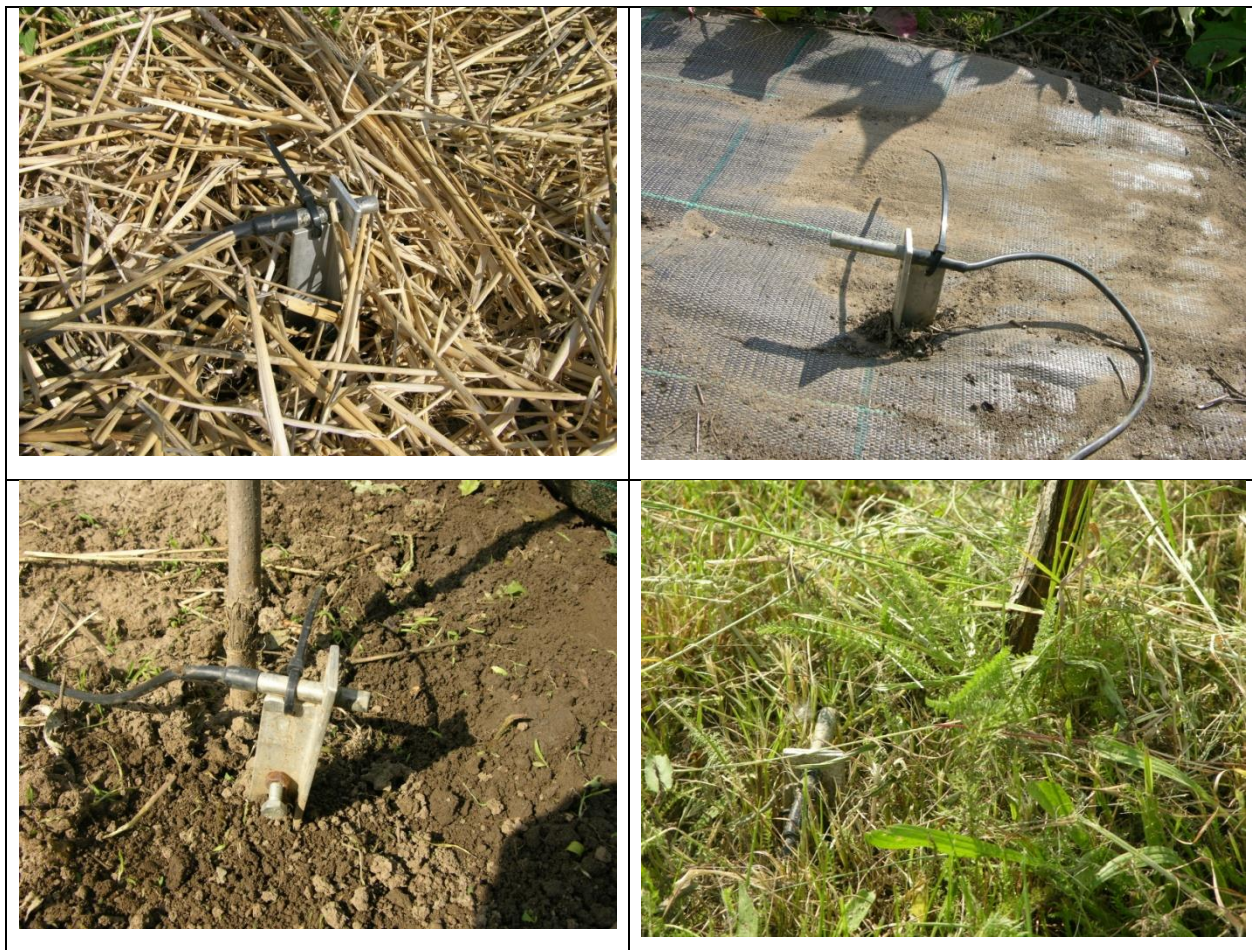
Fig. 2 Position of sensors above the different surfaces
