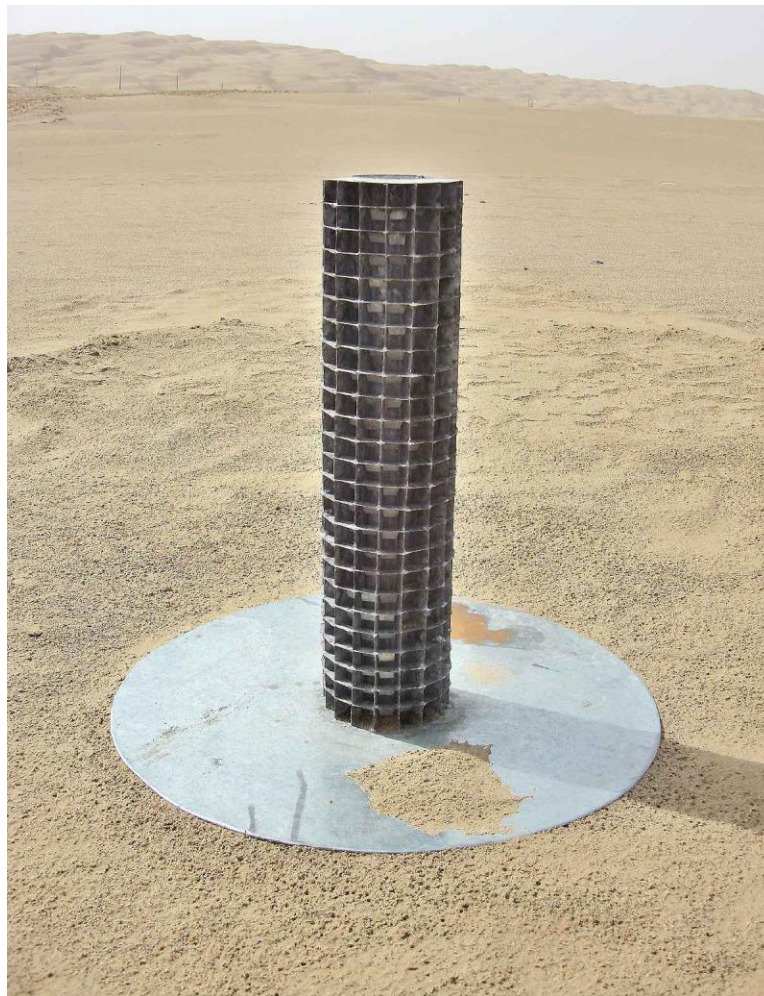
Fig. 1 Bagnold collector (www.sensit.com)
