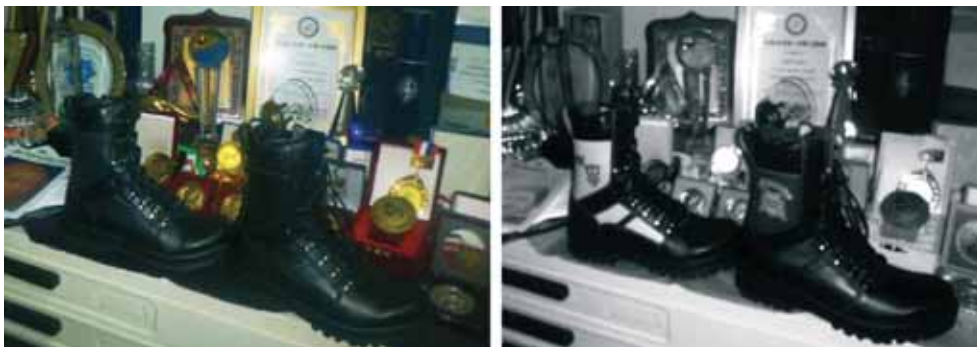
Fig. 16 a,b – Black boots with black dye that responds as white in the Z spectrum
