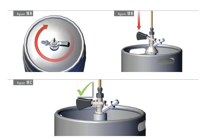
**18.2 Keg Untapping:**Procedure for untapping a keg using an S-system keg coupler:
