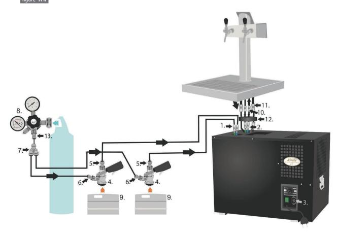
**RECOMMENDATION:** Only use quick couplings to connect beverage hoses. For the connection of tubes for the beverage use only fittings and clips specified by the supplier. Use a calibrated hoses.
