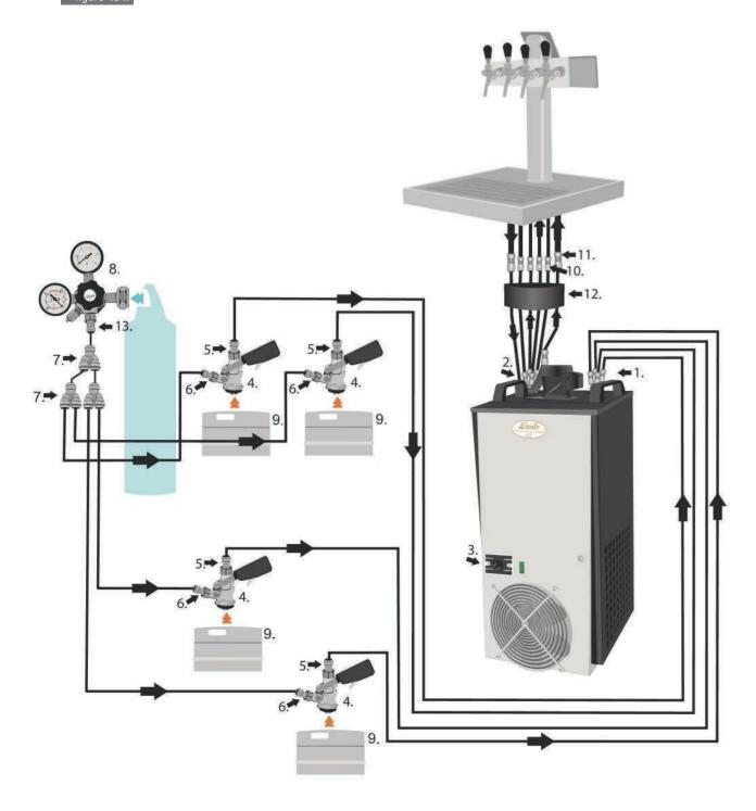
**WARNING:** Check that all joints are sufficiently leak-tight after connection.
