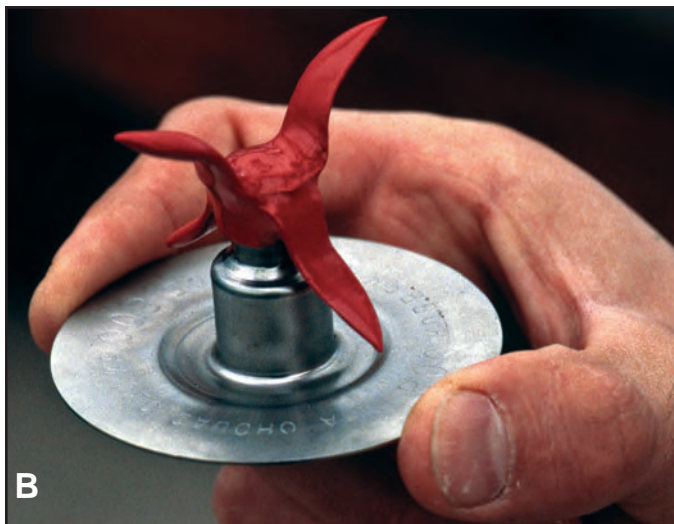
Figure 2.12 —Small batches of berries or other fleshy fruits can be cleaned with a modified food processor (A). Coating the impeller blades with plastic or tape (B) prevents seed damage.
