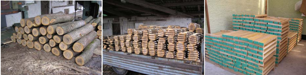
Figure 1. Small-sized roundwood, sawn boards, dimension stock and raw parquet staves
